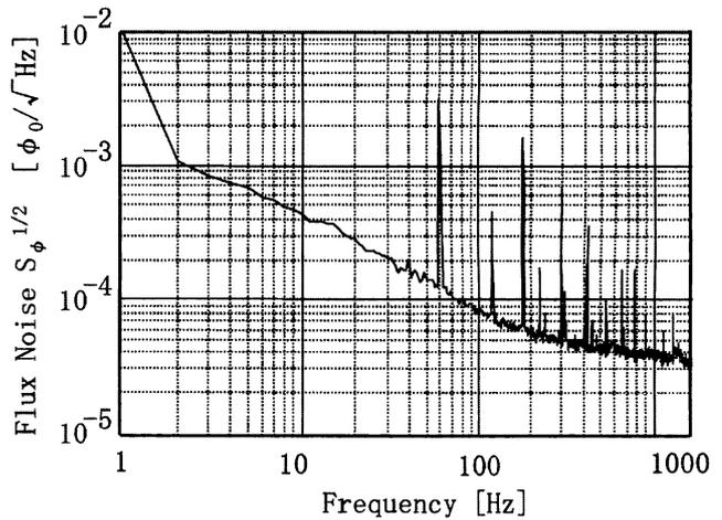
**Figure 6.** Flux noise of magnetometer with needle. The noise with needle was  $80 \mu\phi_0/\text{Hz}^{1/2}$  at 100 Hz and  $36 \mu\phi_0/\text{Hz}^{1/2}$  in the white noise region. Excess  $1/f$  flux noise, which may be generated by the thermal activated hopping of vortices trapped during cooldown, was observed.
