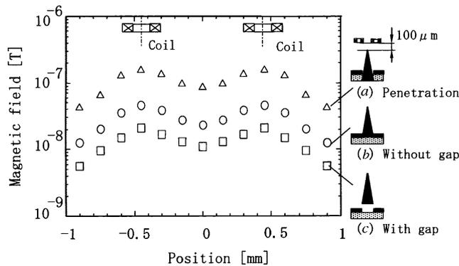
**Figure 2.** Effect of the position of the needle in simulation. Two peaks, one at the position of each field coil, were observed in all the cases. The field density in the case of (a) is the largest and one order of magnitude larger than that in the case of (c).
