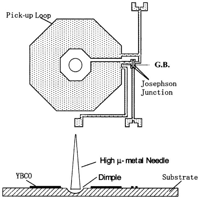
**Figure 5.** Schematic drawing of a directly coupled dc SQUID. The SQUID inductance was 40 pH in the calculation. The outer and inner diagonal dimensions of the pick-up loop were 6.4 mm and 2.2 mm, respectively. The substrate at the centre of the pick-up loop was machined so that a 100–200  $\mu\text{m}$  deep dimple is created for the needle space.
