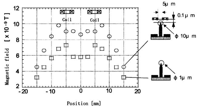
**Figure 3.** Effect of the size of the top of the needle in simulation. The peaks of the field with the needle of a diameter of  $1 \mu\text{m}$  are sharper than those with a diameter of  $10 \mu\text{m}$ . This result suggests that the needle with smaller top shows a better space resolution.
