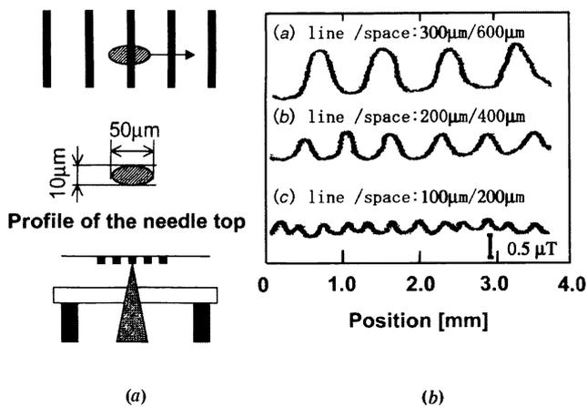
**Figure 7.** Results of the scanning. (a) Schematic drawing of the scanning configuration and (b) the output signal of the SQUID when laser-printed bar patterns were scanned. The finest pattern we prepared was a line width of  $100 \mu\text{m}$  and a spacing of  $200 \mu\text{m}$  between lines.
