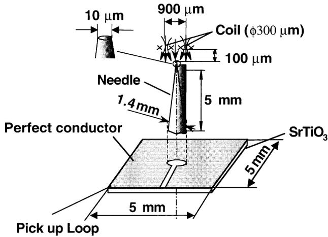
**Figure 1.** Model of the simulation. One set of small field coils with a separation of  $900 \mu\text{m}$ , which generated a magnetic field of  $10 \text{ mA m}^{-1}$ , was positioned above the pick-up loop. The relative position of the set of coils and the pick-up loop was varied by a step of  $150 \mu\text{m}$  in this simulation. The separation between the top of the needle and the coil was kept constant at  $100 \mu\text{m}$ .
