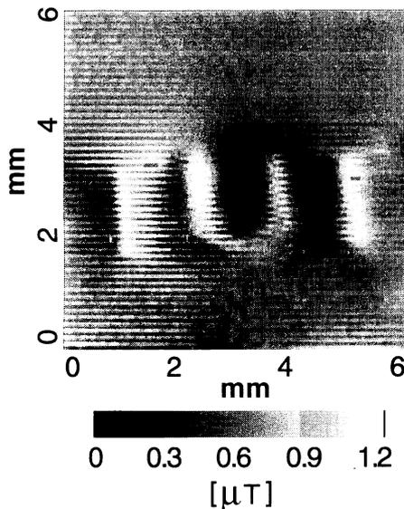
**Figure 8.** Two-dimensional magnetic field image of the printed pattern of the characters TUT.
